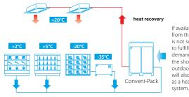
If available heat from the cabinet is not sufficient to fulfill the demand from the shop, the outdoor unit will also operate as a heat pump
