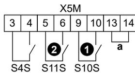
a Jumper (factory-mounted). If you also connect a safety thermostat (Q4L), replace the jumper with the safety thermostat wires.
