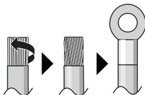
**Use the following methods for installing wires:**
