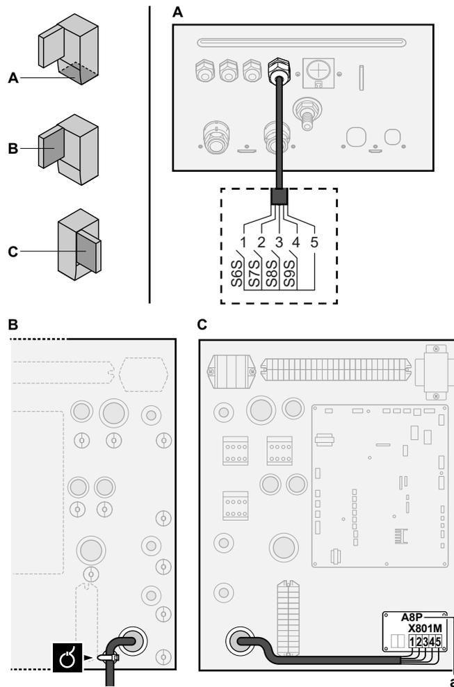
a Installation of EKRP1AHTA is required.
