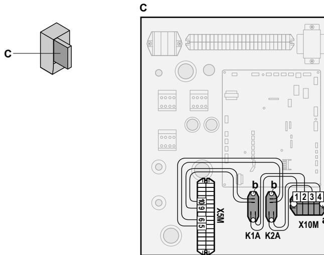
2 Connect the low voltage wiring as follows:
