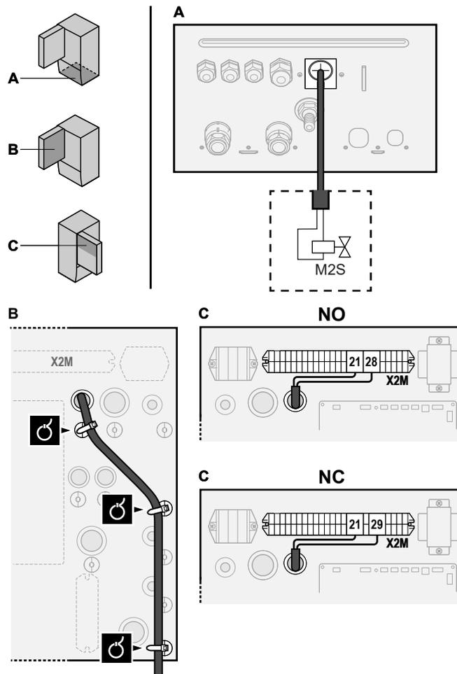
3 Fix the cable with cable ties to the cable tie mountings.
