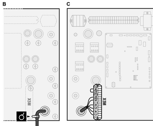
2 Fix the cables with cable ties to the cable tie mountings.
