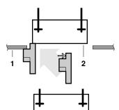
Apply the long side of the installation guide in case of installation with fresh air intake kit
